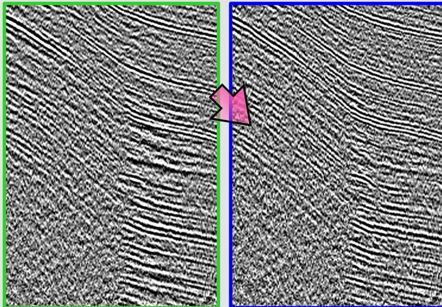
The result is better details & more continuity on the data (middle vs. left) and an increased frequency content of up to 6 dB.
