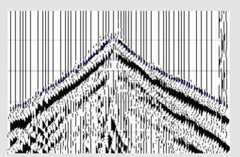
Thorough first break picking leads to accurate statics models and **enhanced imaging**
