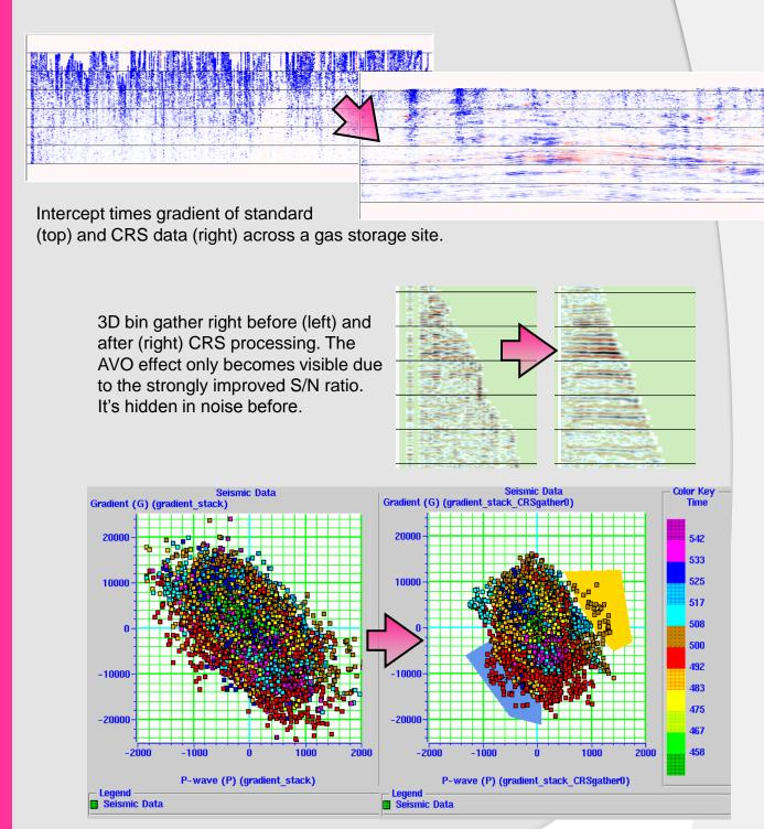
AVO crossplot before (left) and after (right) CRS processing. The wet trend is compacted and the hydrocarbons are seperated from the wet trend.
