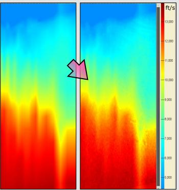
Stacking velocity model before (left) and after (middle) CRSplus auto update. The difference plot (right) shows subtle structure-related details detected by the autoupdater.
