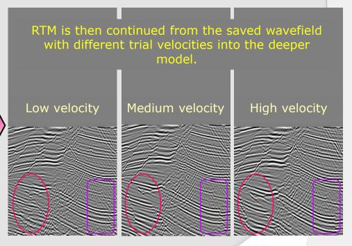
In the RTM trial zone, the best structural focussing and CRP gather flatness is picked at selected locations and at the corresponding trial velocities. These locally accepted trial velocities are evaluated by a velocity update algorithm.
